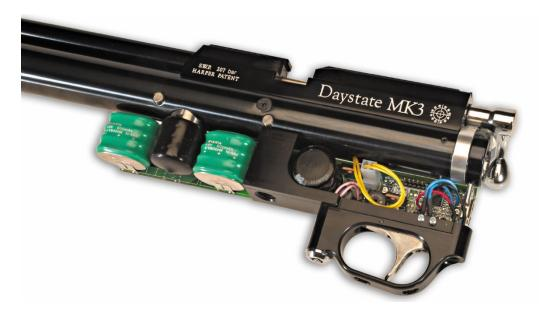
MK3 RT (Regulated Thumbhole) models were fitted with an external regulator which because of its position necessitated the battery stacks being separated to fit.
