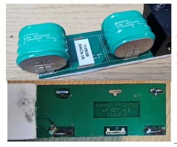
Remove the two soldered in batteries by turning over the board, removing the insulation, and with a soldering iron, heat up the push in battery pins so the batteries will fall free and clear of the board.
