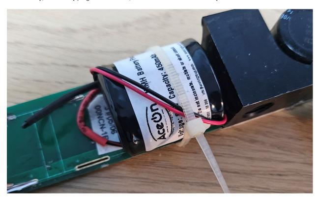
The plug in battery can then be affixed to the board using a zip lock connector.
