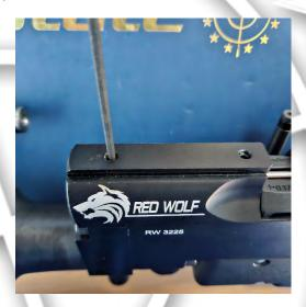
2. Once the barrel is removed, screw in the barrel locating screws until the screws are flush with the breech block.
