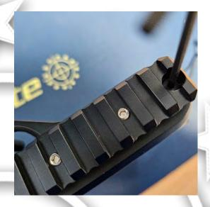
5. side in place the rear picatinny section, aligning as shown. Tighten the 3 silver rail screws.
