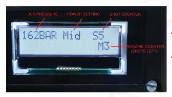
The Red Wolf's GCU 2.0 electronic system provides the user five resettable settings:
