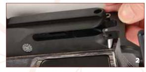
• Use a 2mm hex tool to loosen (but not remove) the two, small hex-head bolts visible through the exposed breech block opening. A quarter turn is all that is needed (3)
