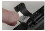
turret. In this instance, place a sliver of silver foil, folded to a maximum thickness of 0.3mm, between the scope and the mount's lower cradle. Do not over-pack the mount, however, as this may damage the scope
