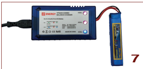
7 When charging, and battery is between 80% & 90%, cell one and two will light as per photo
