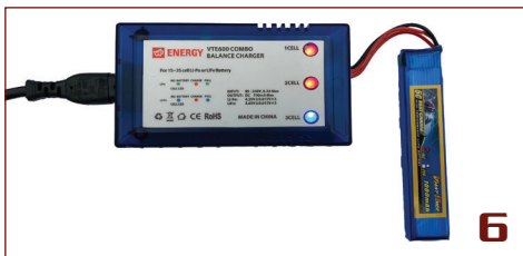
6 When charging, and battery is below 80%, cell one and two will light as RED as per photo
