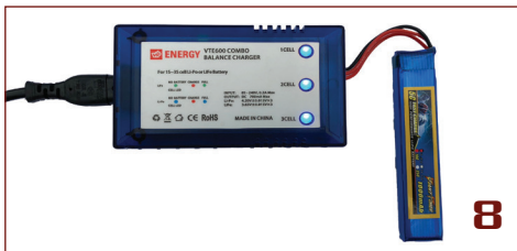
8 When charging completed, all LED's will be a solid BLUE.
