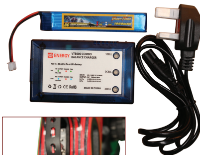
7 When charging, and battery is between 80% & 90%, cell one and two will light as per photo
