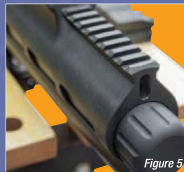
Figure 5: Caution, over adjustment on horizontal may prevent the beam exiting the aperture
