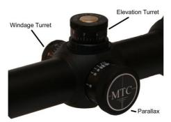
Access to the adjustment is gained by removing the covering caps. The adjusters are finger adjustable. The bullet strike is marked with up/ down (top turret) and left/right (side turret), i.e. if you want the bullet to go higher, turn anti-clockwise in the direction marked "up"
