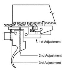
**3RD ADJUSTMENT:** This screw will adjust the first stage travel. Turning it anti-clockwise will increase the travel and clockwise will decrease the travel.
