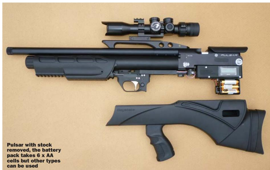
Pulsar with stock removed, the battery pack takes 6 x AA cells but other types can be used
