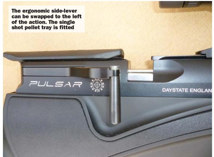
The ergonomic side-lever can be swapped to the left of the action. The single shot pellet tray is fitted
