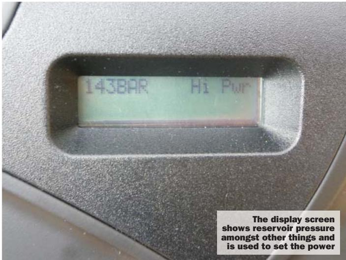
The display screen shows reservoir pressure amongst other things and is used to set the power
