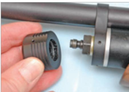
A push-pull fit valve cover keeps things simple, neat and clean
