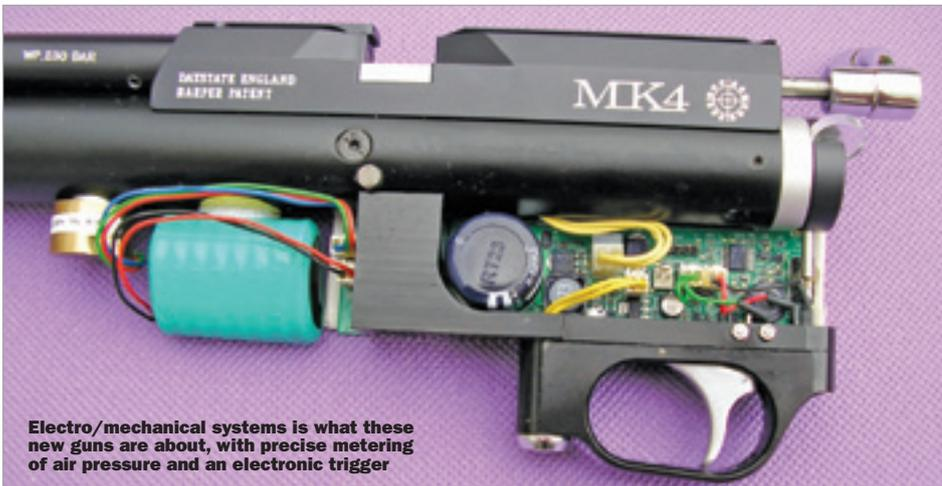
Electro/mechanical systems is what these new guns are about, with precise metering of air pressure and an electronic trigger
